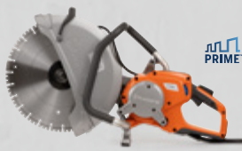
HUSQVARNA K 7000 RING 230/400 V, 5.5 kW (3-phase) / 3 kW (1-phase), 13.1/12.4 kg, blade size 350/425 mm, cutting depth 270/325 mm.
