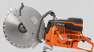
HUSQVARNA K 1270 119 cc, 5.8 kW, 13.3/13.7 kg, blade size 350/400 mm, cutting depth 118/145 mm.
